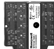
**NOTE** - The Free Cooling default setting for outdoor air temperature sensor is 55°F.
