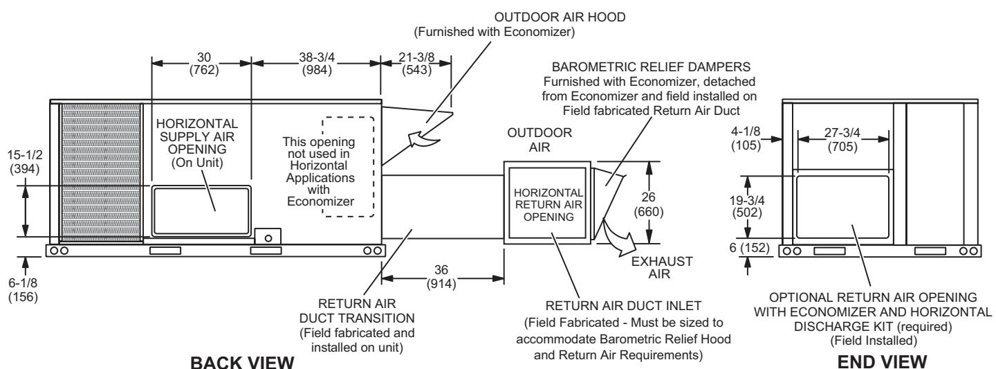
**NOTE** - Return Air Duct and Transition must be supported.
