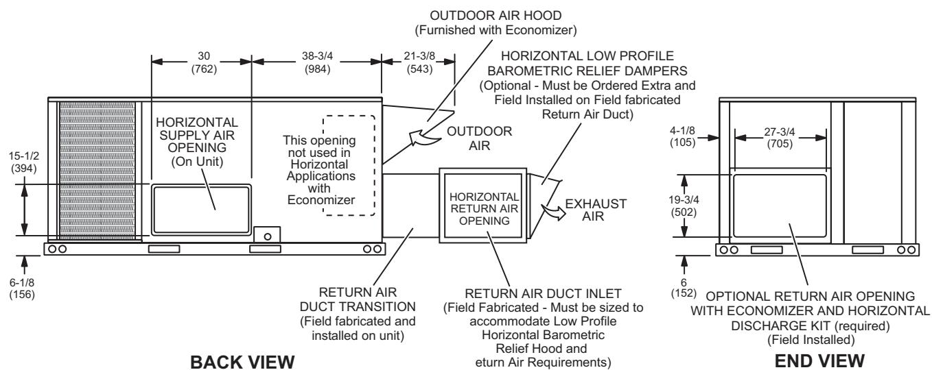
**NOTE** - Return Air Duct and Transition must be supported.
