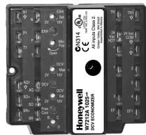
**NOTE:** The Free Cooling default setting for outdoor air temperature sensor is 55°F.
