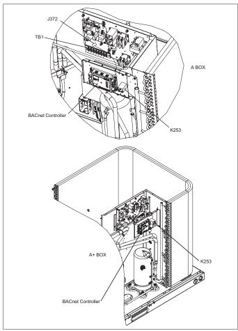
Figure 5. Landmark A- and A+-Boxes
