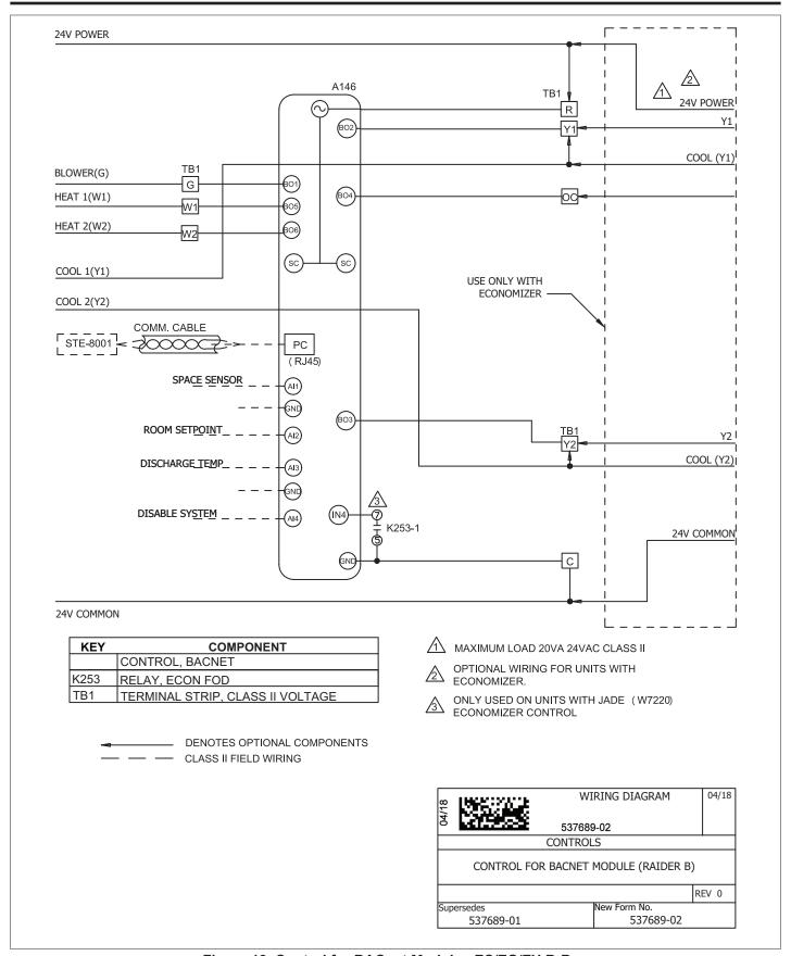
Figure 18. Control for BACnet Module - ZC/ZG/ZH B-Box
