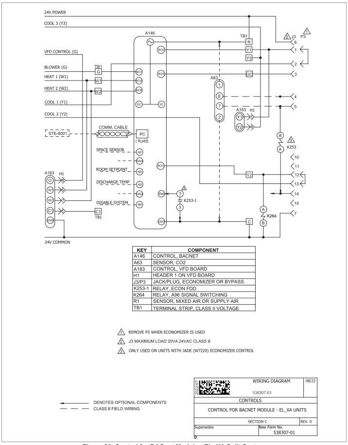
Figure 20. Control for BACnet Module - EL\_XA Split System
