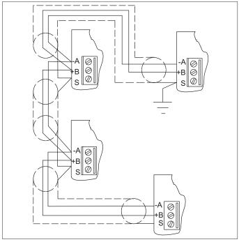
Figure 1. MS/TP Network Wiring
