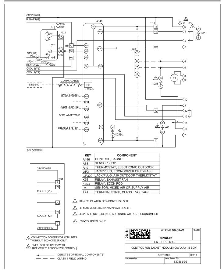
Figure 16. Control for BACnet Module - KD A-, A+- and B-Box (CAV)
