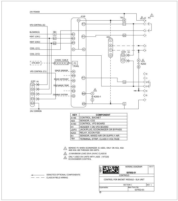
Figure 19. Control for BACnet Module - ELA Split System
