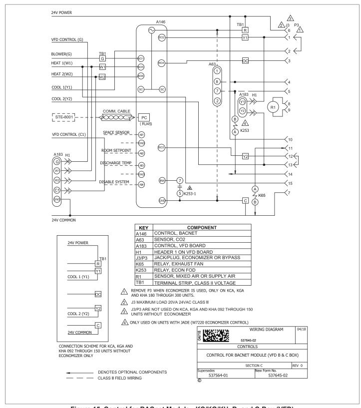
Figure 15. Control for BACnet Module - KC/KG/KH, B- and C-Box (VFD)
