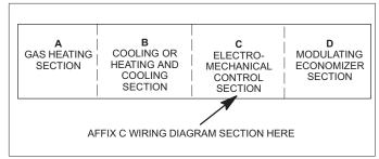
Figure 13. Affixing System Wiring Diagram
