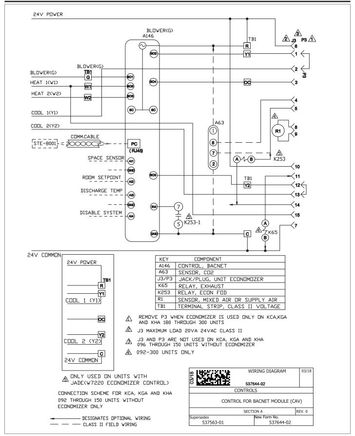
Figure 14. Control for BACnet Module KC/KG/KH A-, A+-, B- and C-Box (CAV)
