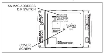
Figure 10. BACnet MAC Address Dip Switches Location (S5)
