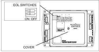
Figure 3. BACnet End-of-Line Switches (S3)
