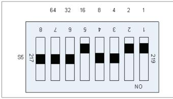
Figure 11. BACnet MAC Address Dip Switches
