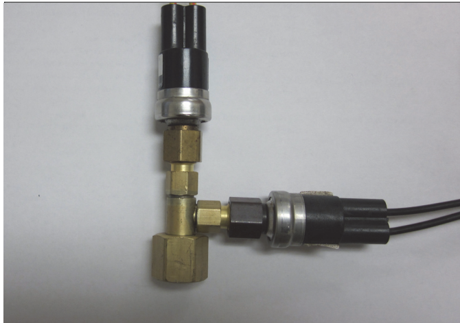
Figure 1. Both Switches Installed on the Tee. Tee Installed on the Suction Line.
