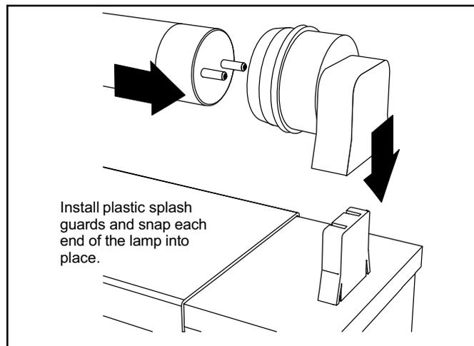
**Figure 2. Installing Lamp in Holder Clips**
