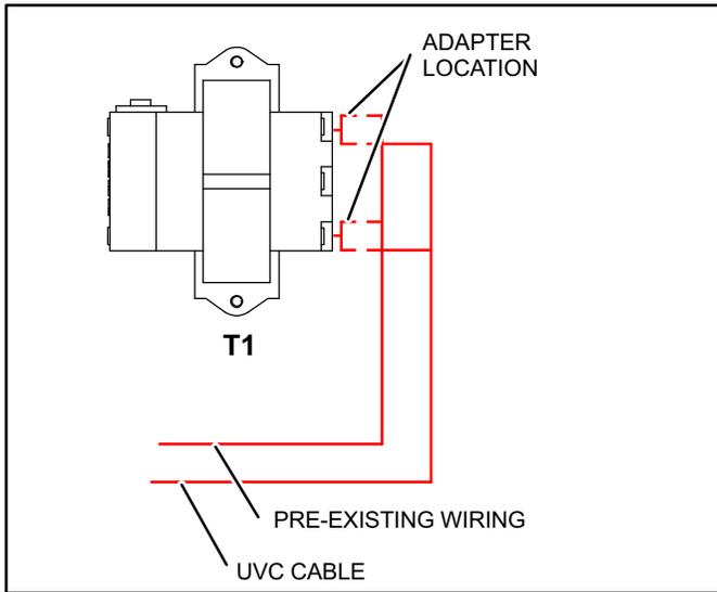
**Figure 5. Connect cable to transformer T1 (230 Volt units)**
