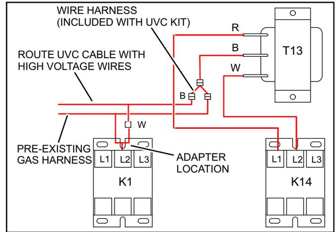
**Figure 7. Connect cable to transformer T13 (575 Volt units)**
