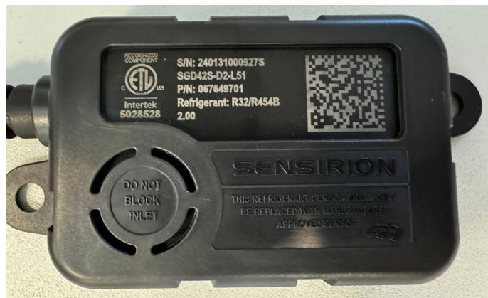
FIGURE 14. Example of Clear, Unobstructed Sensor Inlet
