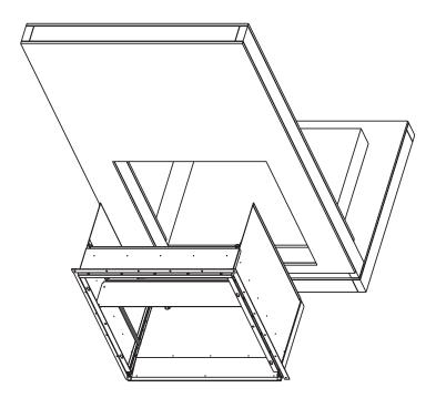
Fig 5: Installing Wall Sleeve from Outside of Building
