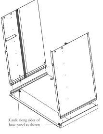
Fig 9: Caulk Sealing Wall Sleeve Base
