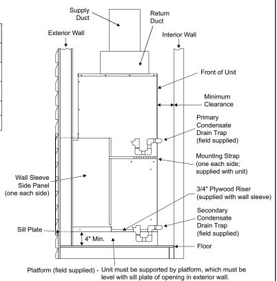
Fig 3: Minimum Clearances - MHP/MCE Units
