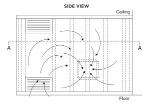
If wall space is not to be used for return air passage, full 2-1/2 or 3 in. thickness fiberglass insulation should be used.
