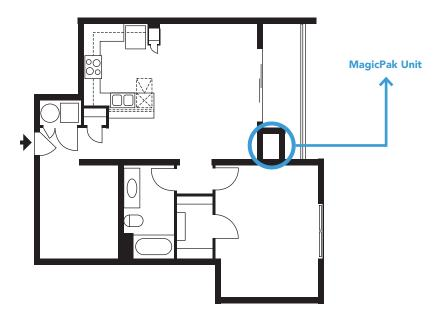
Figure 1: Condominium with MagicPak on exterior wall
