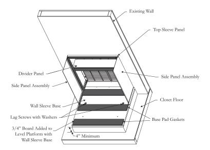
**NOTE:** The platform base must be sized to support the full length and width of the bottom of the unit and constructed so that it is level with the sill plate of the wall opening.
