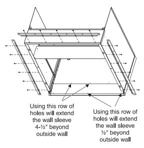
Fig 6: Flashing Angles
