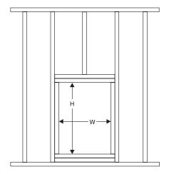
Fig 11: Wall Opening in Frame Wall
