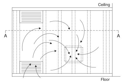
If wall space is not to be used for return air passage, full 2-1/2 or 3 in. thickness fiberglass insulation should be used.
