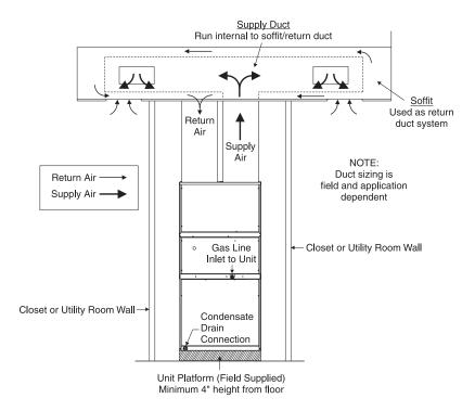
Fig 14: Concentric Supply and Return Duct System for MGE MagicPak Unit
