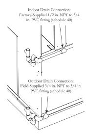
Fig 19.: MCE/MHP Condensate Drain Connections
