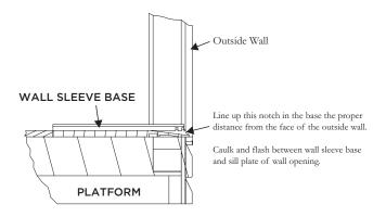
Fig 8: Positioning Wall Sleeve Base
