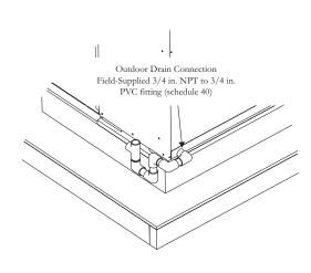
Fig 18: MGE Condensate Drain Connection
