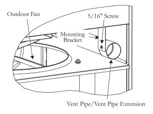
Fig 16: Locating MagicPak MGE Vent Pipe Extension
