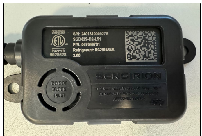
FIGURE 10. Example of Clear, Unobstructed Sensor Inlet
