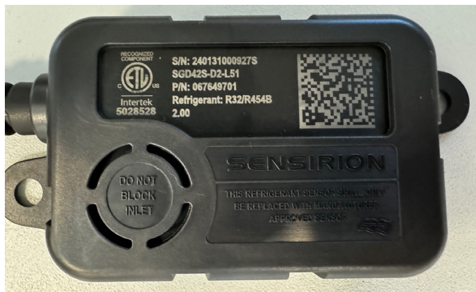
FIGURE 12. Example of Clear, Unobstructed Sensor Inlet
