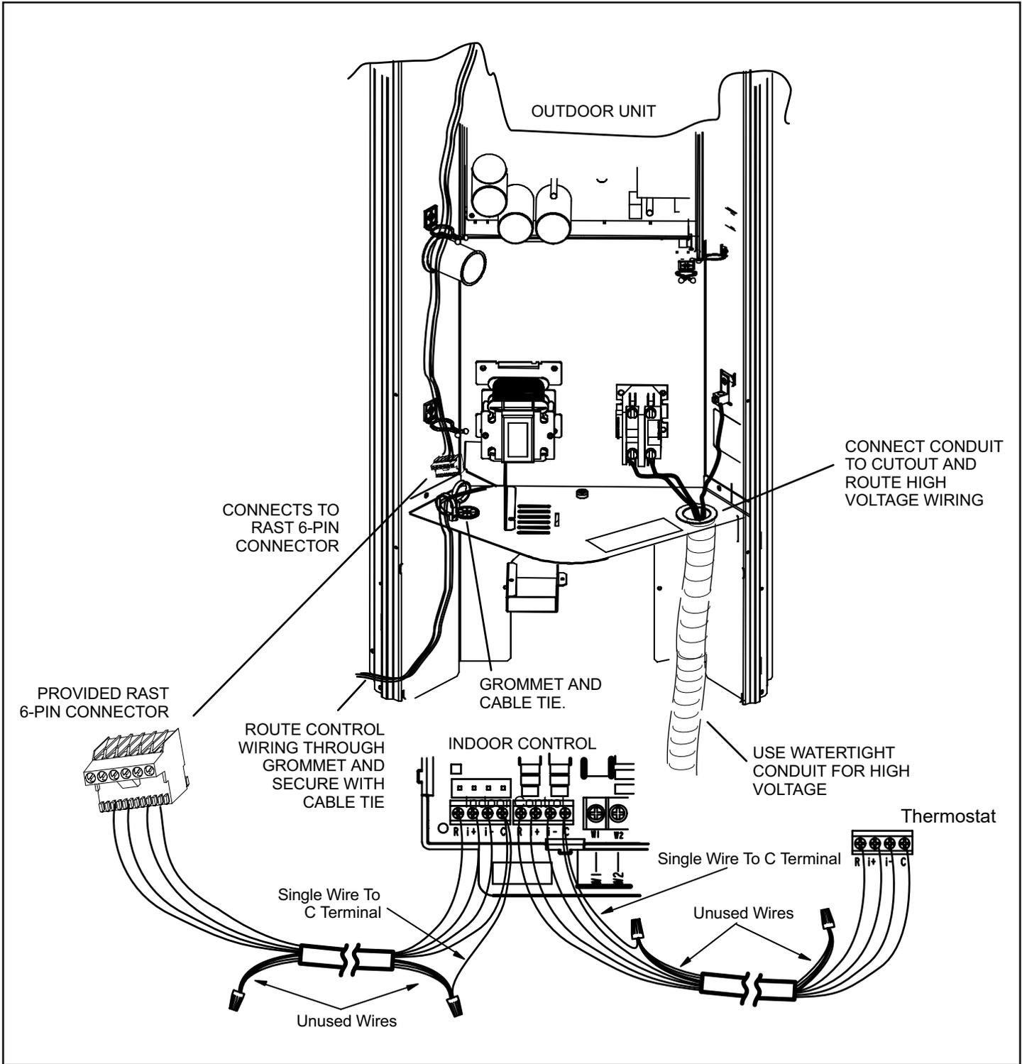
Figure 6. Control Wiring
