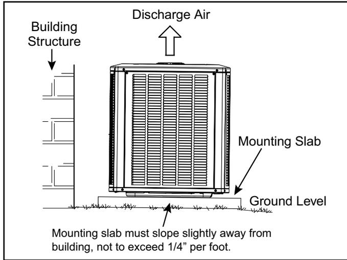
**Figure 1. Slab Mounting**
