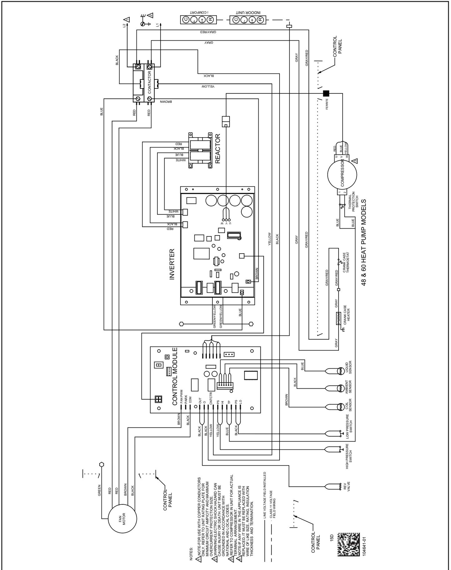
Figure 9. A/C Single Phase Wiring Diagram - 48 & 60 Models
