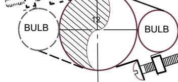
ON 7/8" AND LARGER LINES, MOUNT SENSING BULB AT EITHER THE 4 OR 8 O'CLOCK POSITION.
