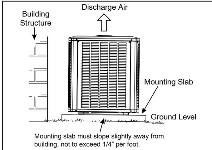
**Figure 1. Slab Mounting**
