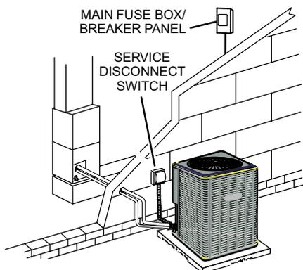
**NOTE** - Units are approved for use only with copper conductors. Ground unit at disconnect switch or connect to an earth ground.
