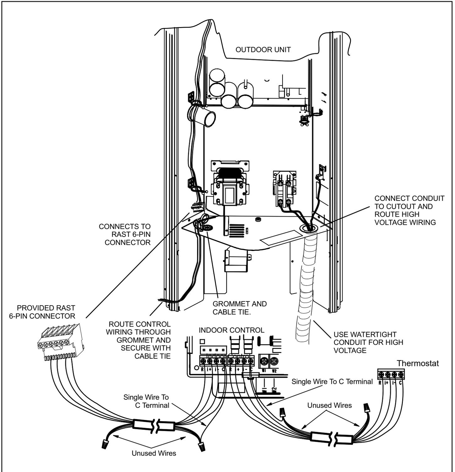
**Figure 7. Control Wiring**
