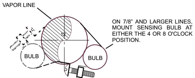
**NOTE** - NEVER MOUNT THE SENSING BULB ON BOTTOM OF LINE.
