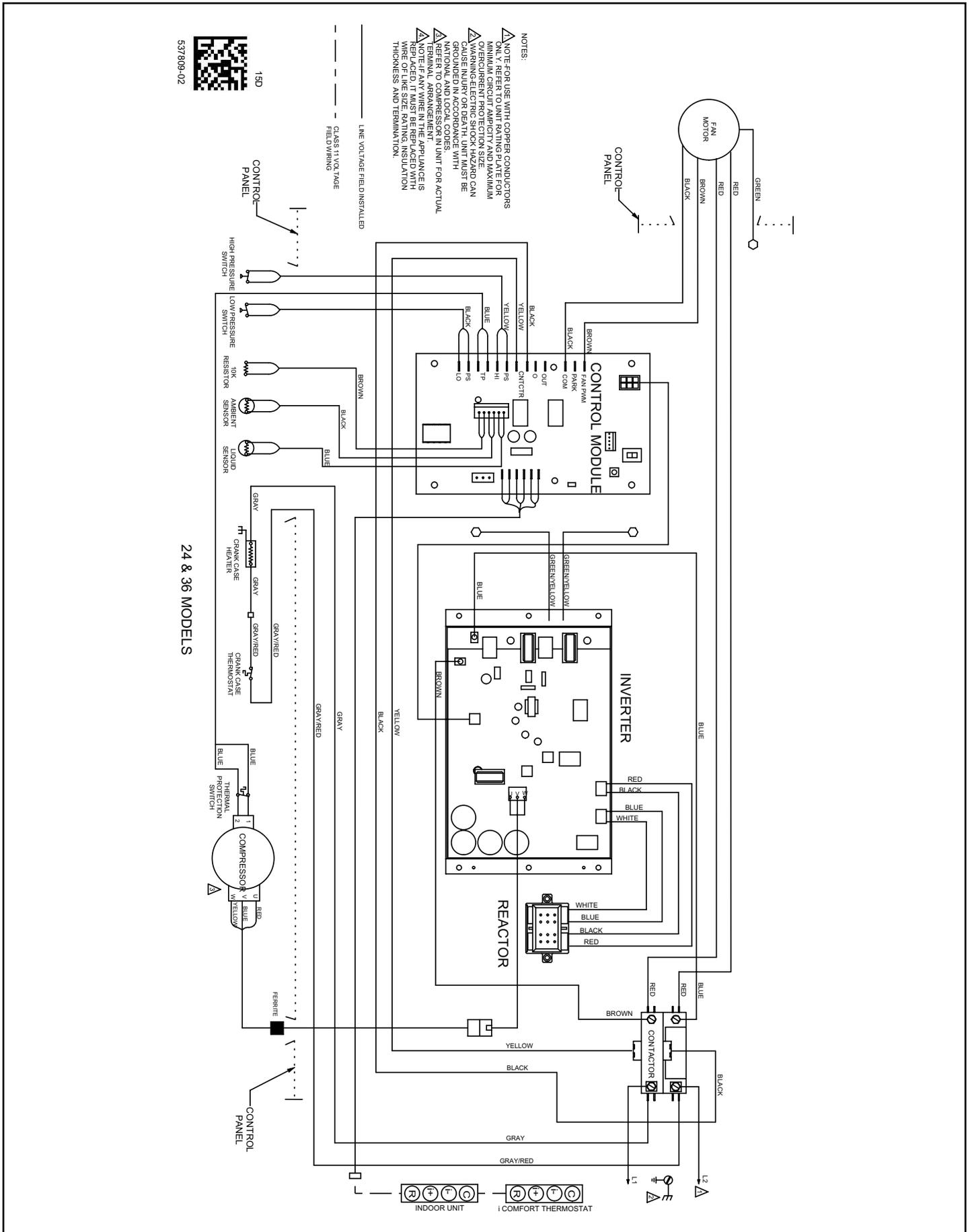
Figure 9. A/C Single Phase Wiring Diagram - 24 & 36 Models
