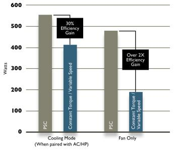
Variable-Speed and Constant-Torque air handlers are up to 30% more efficient than PSC units.
