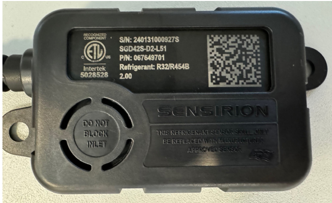
FIGURE 11. Example of Clear, Unobstructed Sensor Inlet
