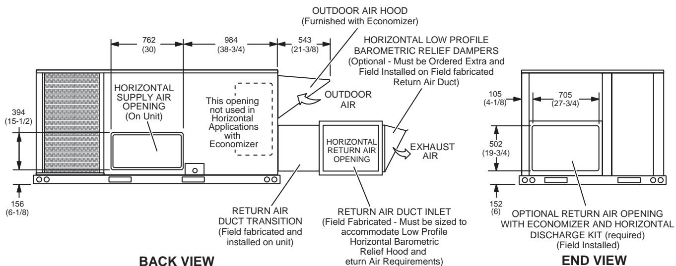
**NOTE** - Return Air Duct and Transition must be supported.
