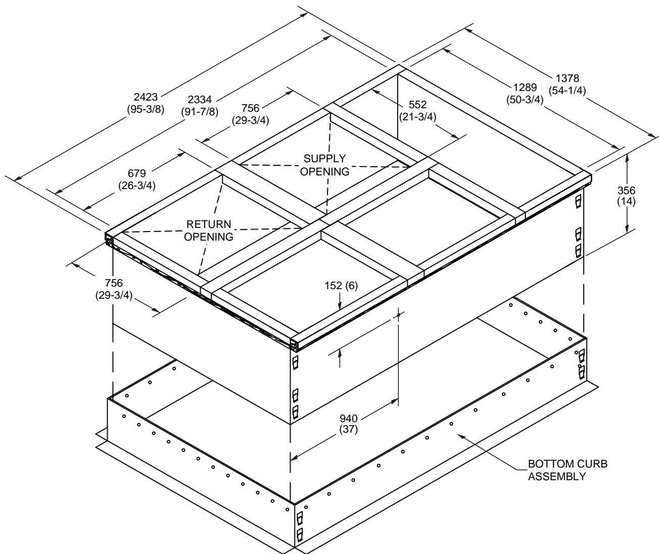
NOTE - Maximum slope pitch is 19 mm per 305 mm (3/4 in. per 1 foot) in any one direction.
