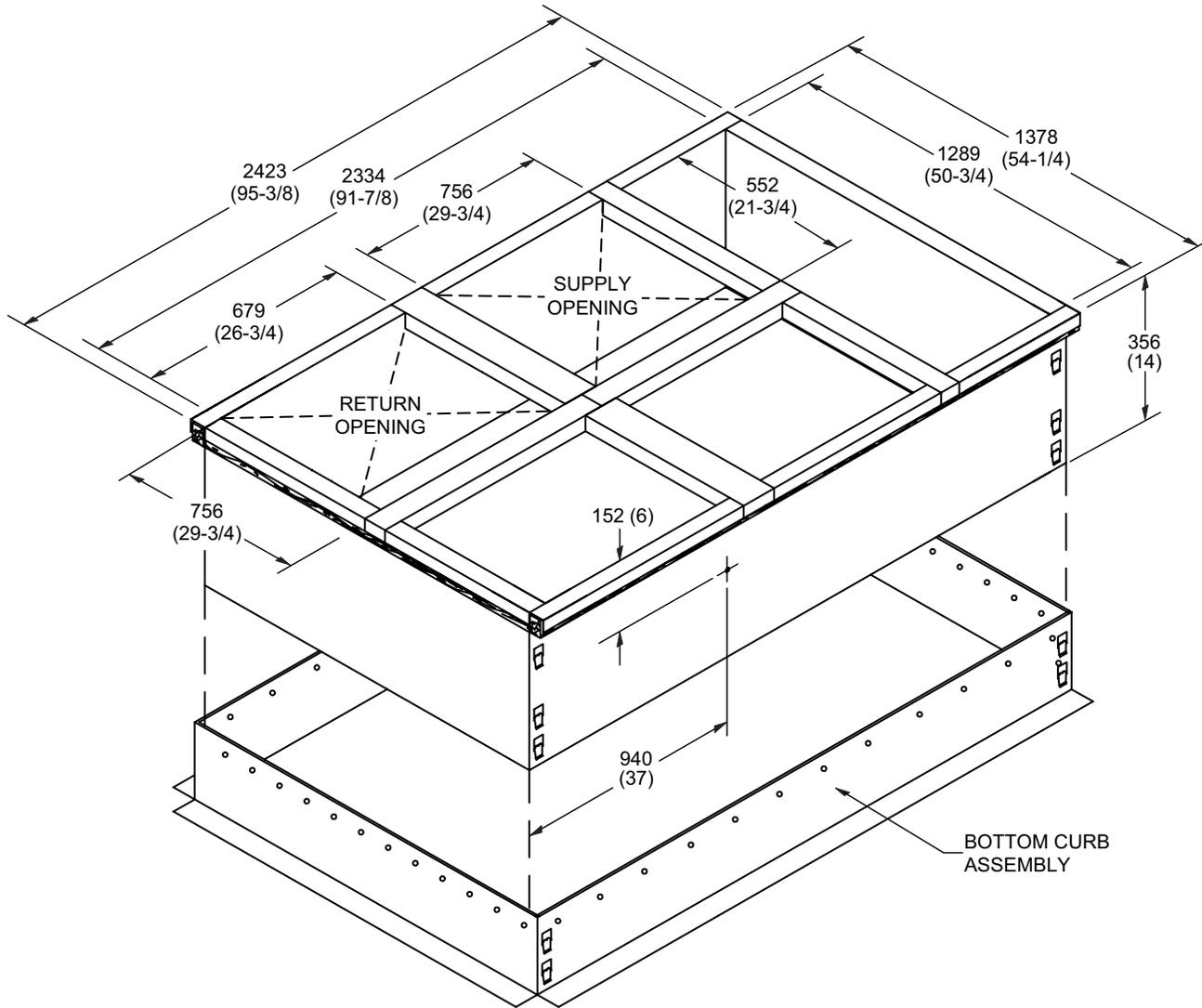
NOTE - Maximum slope pitch is 19 mm per 305 mm (3/4 in. per 1 foot) in any one direction.
