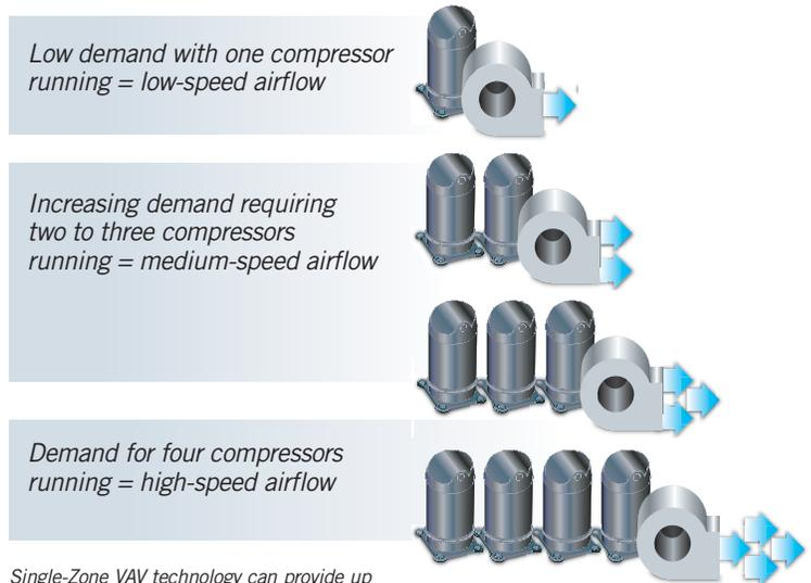
Single-Zone VAV technology can provide up to seven levels of airflow for four-compressor systems.
