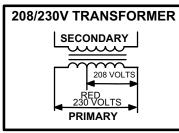
mary voltage taps as shown in figure 3, while 460 (G) and 575 (J) voltage transformers use a single primary voltage tap.
