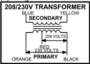
shown in figure 3, while 460 (G) and 575 (J) voltage transformers use a single primary voltage tap.
