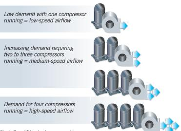
Single-Zone VAV technology can provide up to seven levels of airflow for four-compressor systems.
