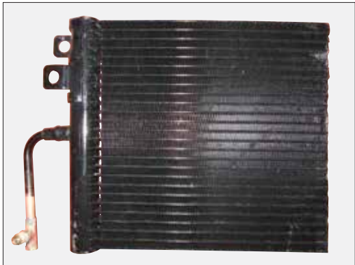
Figure 5: E-Coated Sample Before Testing
