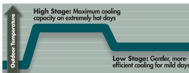
With its two-stage design, the 4SHP18LT makes the distinction between mild and extremely hot or cold days, using only the energy necessary to keep you comfortable.
