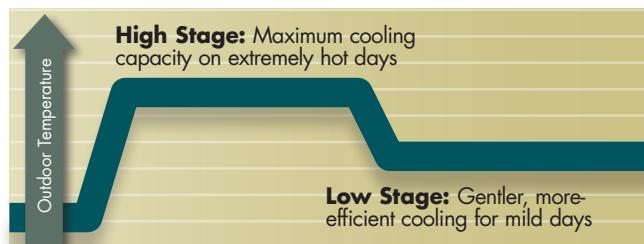
With its two-stage design, the 4SCU16LT makes the distinction between mild and extremely hot days, using only the energy necessary to keep you comfortable.
