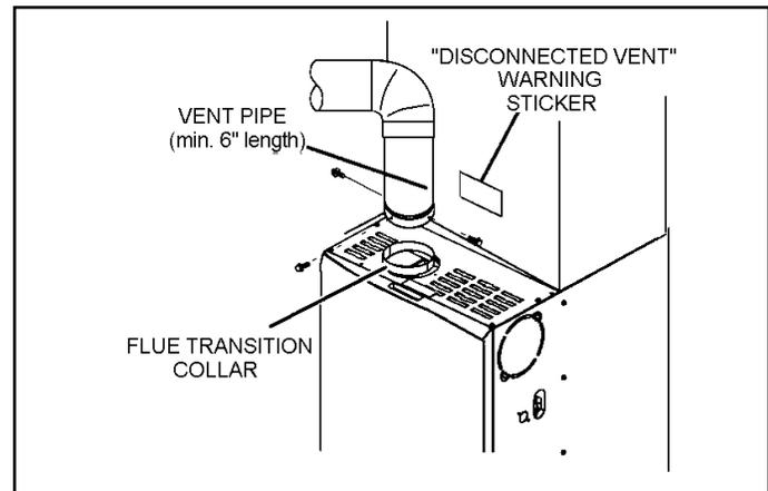
**Figure 22. Vent Connection**
