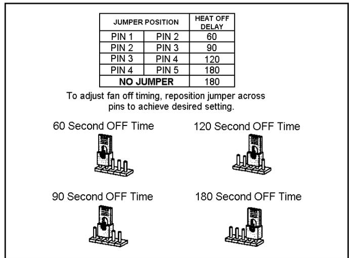
**Figure 35. Heat Fan Off Time in Seconds**
