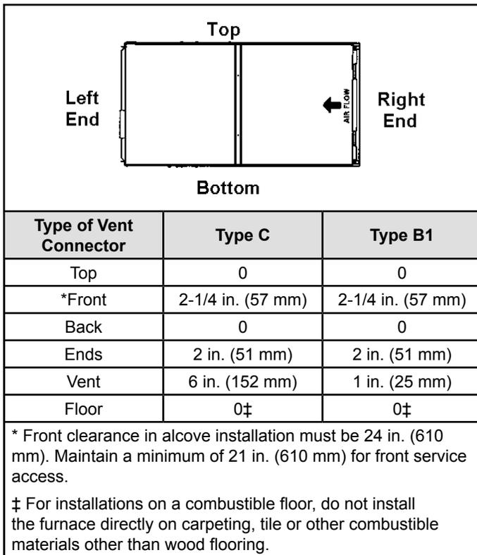
**Figure 10. Horizontal Application Installation Clearances**
