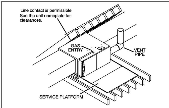
**Figure 13. Horizontal Application Unit installed on Platform**
