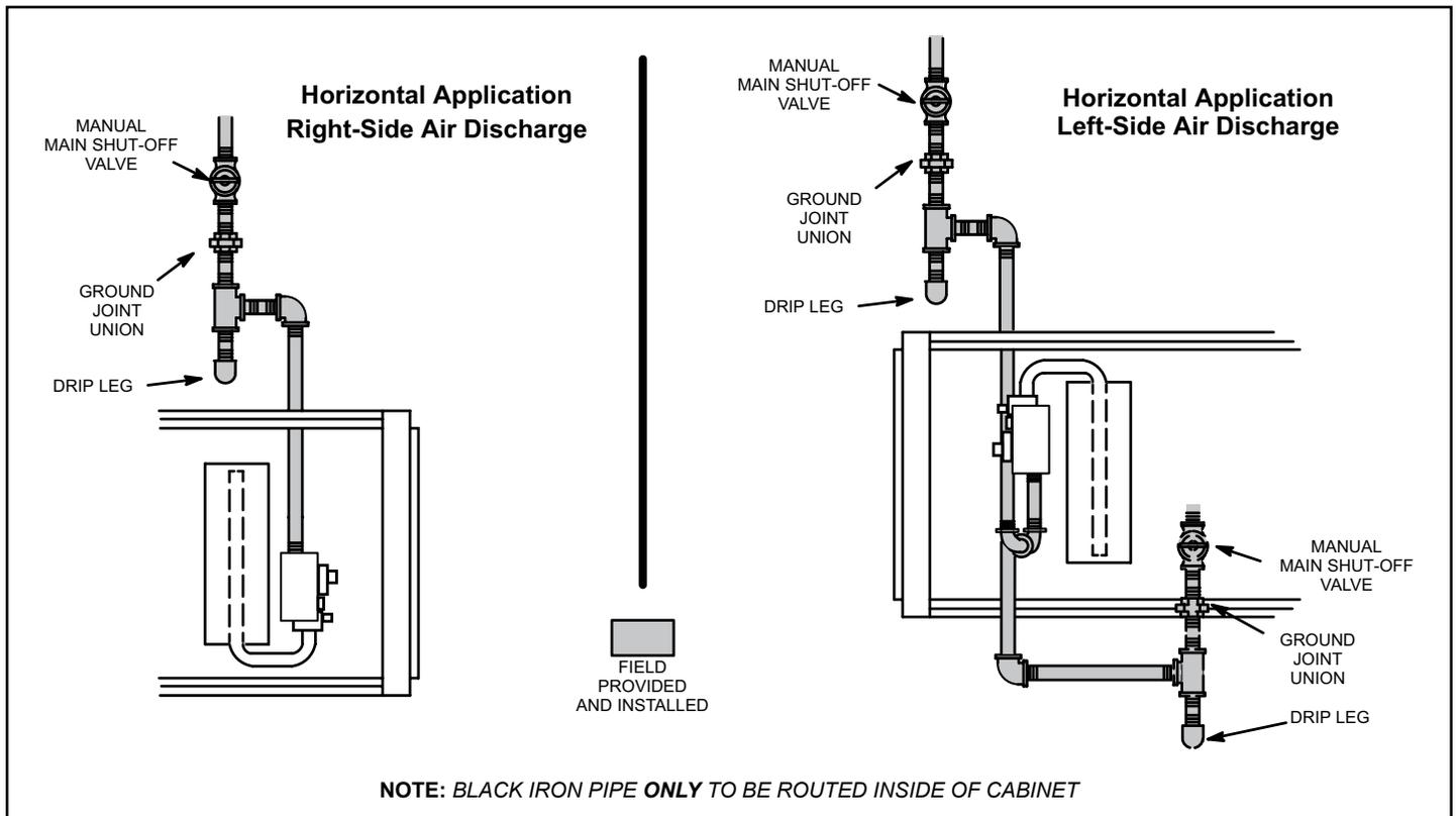
**Figure 25. Possible Gas Piping Configurations - Horizontal Applications**
