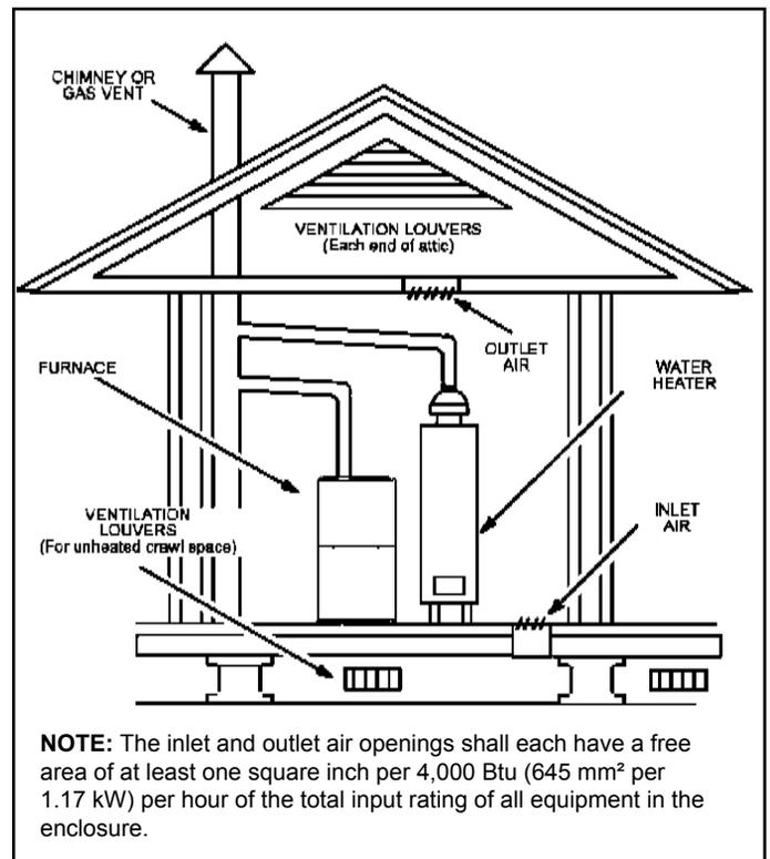
**Figure 3. Equipment in Confined Space - All Air from Outside
