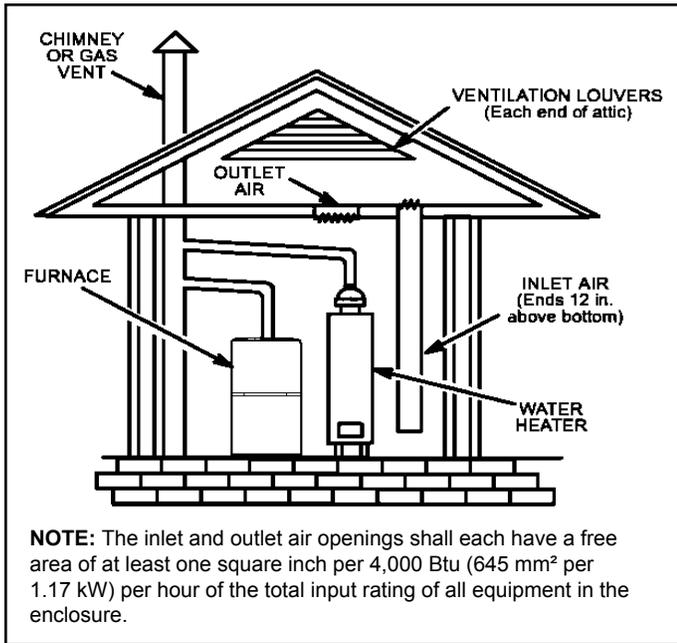
**Figure 4. Equipment in Confined Space - All Air from Outside
