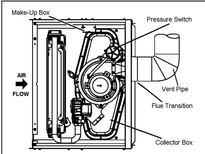
**Figure 21. Horizontal Right Position
