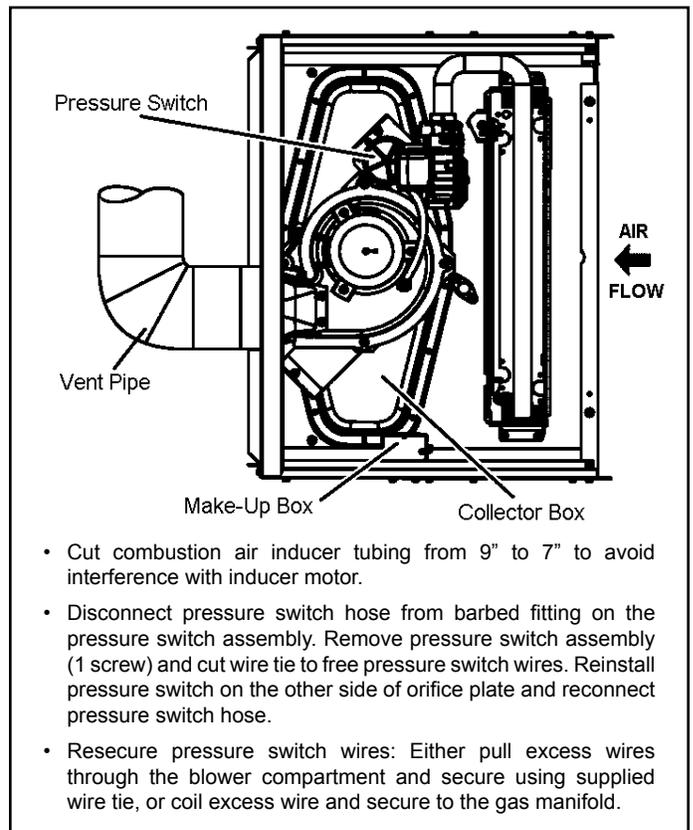
**Figure 19. Horizontal Left Position
