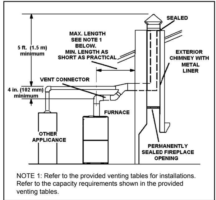
**Figure 23. Common Venting Using Metal-Lined Masonry Chimney**
