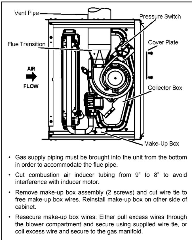
**Figure 20. Horizontal Right Position
