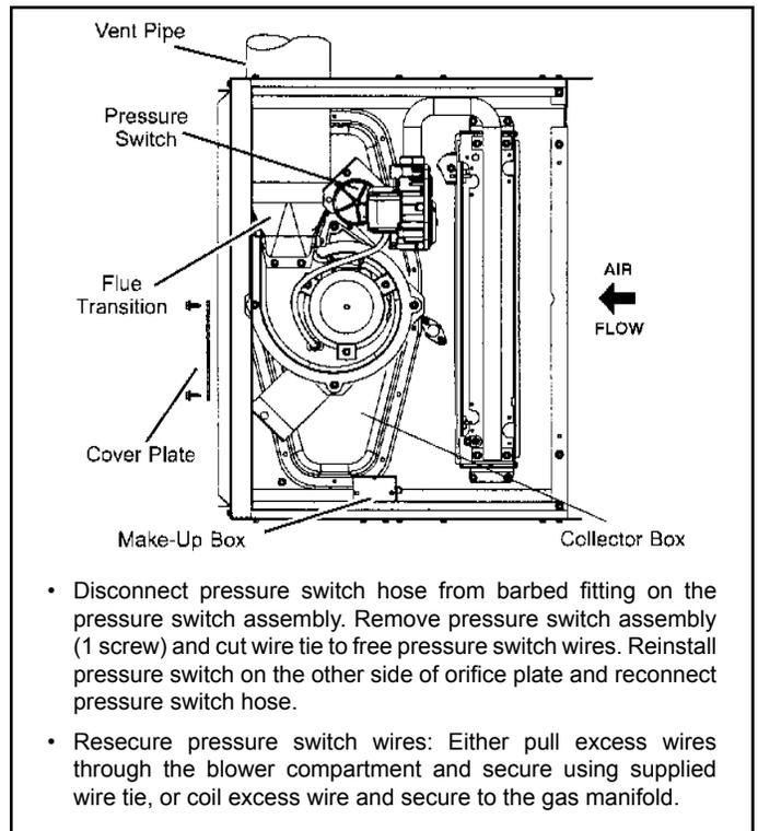
**Figure 18. Horizontal Left Position
