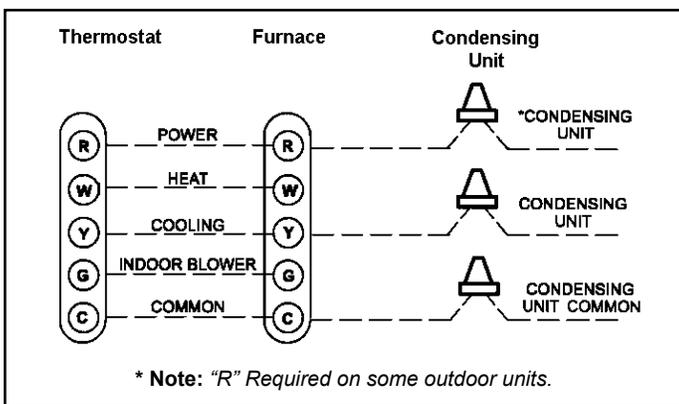
**Figure 32. Condensing Unit Thermostat Designations
