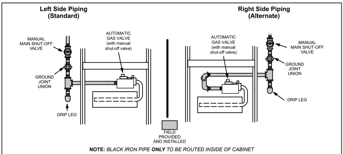
Figure 27. Possible Gas Piping Configurations - Upflow Applications
