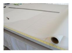
Place the template on the Face Fabric (FF). Using a Chalk Marker, trace around the pattern and cut out the swag.
