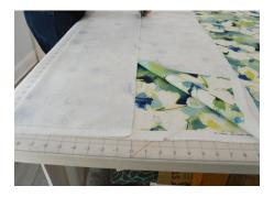
Unfold the fabric of the drapery header. Place the Micro Welt Cord on the fabric with the welt Seam Allowance (SA) at the fold.
