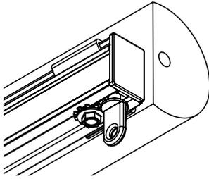
5. The traverse track with the fascia attached will be held in place by the support notch at the end of the bracket and the camlock that locks the track into place. When the track is placed inside the support notch, turn the camlock counter clockwise with a flathead screwdriver to lock the track in place (5A & 5B).
