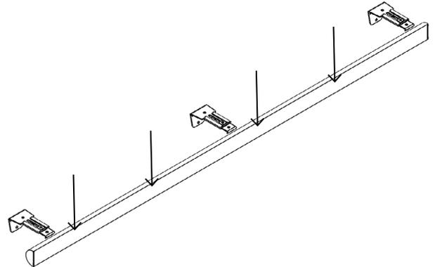
3. Attach the fascia clips at your marked location onto the back of wood fascia as shown below (3A). Align the bottom of the fascia clip with the bottom edge of the wood fascia (3B). Pre-drill the holes with a  $\frac{3}{32}$ " drill to keep the fascia from splitting. Use the screw provided to secure the fascia clip to wood fascia. Do not over tighten.
