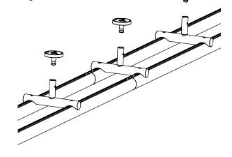
Step 6. Tighten all ceiling mount stems with set screw located close to the ceiling mount cover.
