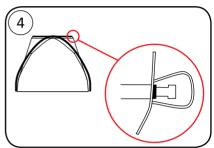
PLACE BROW POLE ON TOP OF "X" POLES AND INSERT INTO GROMMETS
