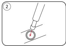
**INSERT POLE TIPS INTO CORNER GROMMETS**
