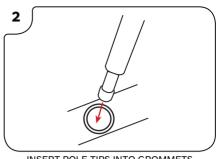
INSERT POLE TIPS INTO GROMMETS
