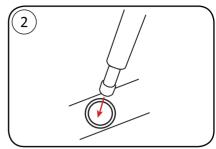
**INSERT POLE TIPS INTO CORNER GROMMETS**
