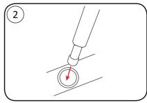
**INSERT POLE TIPS INTO CORNER GROMMETS**
