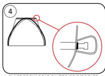
PLACE BROW POLE ON TOP OF "X" POLES AND INSERT INTO GROMMETS
