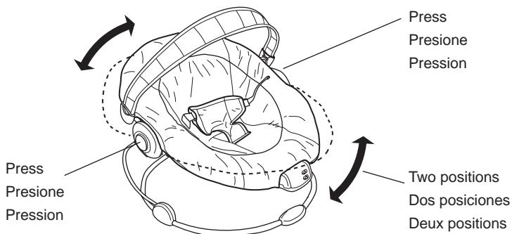
Press the left and right release buttons simultaneously and carefully rotate the frame up or down into the desired position.
