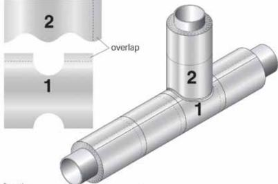
On "tee" sections, make appropriately configured templates of VentureClad, leaving a 1 inch (25 mm) overlap.
