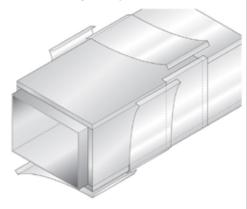
Pre-cut the VentureClad to the required size, plus an additional overlap of 3 inches (75 mm) for each adjoining surface.
