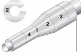
On reduced pipe, apply VentureClad first to surface No.1, overlapping onto surface No.2. Cut shape No. 2, allowing for 3 inch (75 mm) overlap, and apply to surface No.2, overlapping onto section No.1.
