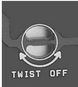
Fig. 1 - PCB Breakout Jumper
