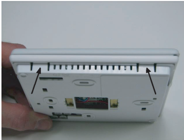
Fig. 3 - Press Tabs to Remove Backplate
