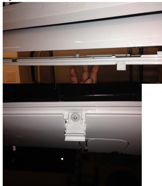
Figure 95: Remove Screws from Bottom Panel
