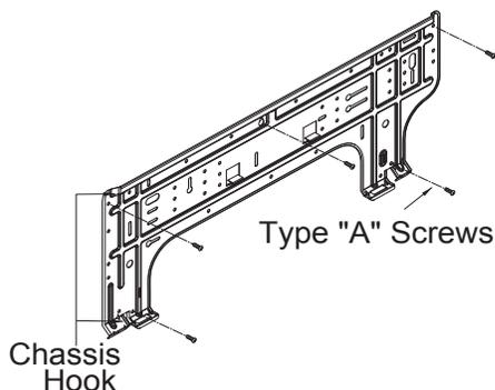
Figure 14: Wall Mount Indoor Unit Installation Plate Dimensions.
