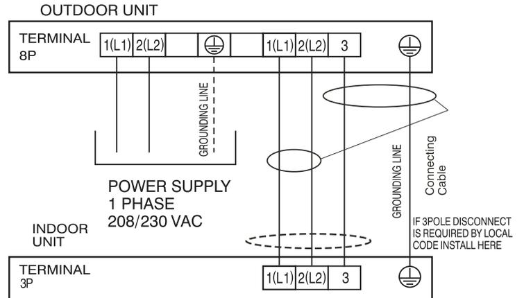
Figure 83: Typical LA240HSV3 Power / Communication System Diagram For Wiring Lengths GREATER THAN 130 Feet.
