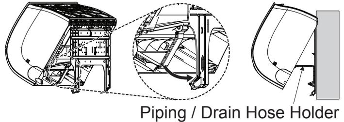
Figure 24: L-bracket Closed (Appearances May Vary Depending on Indoor Unit Model).
