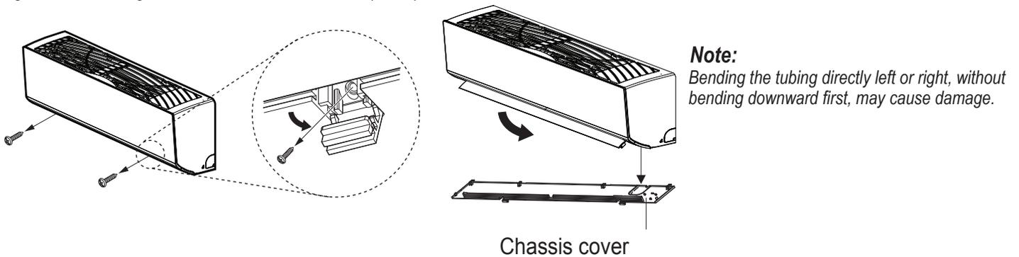
Figure 53: Incorrect: Bending Pipe tubing from Indoor Unit (HSV3).
