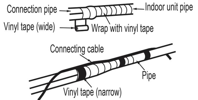
Figure 63: Cutaway of Proper Pipe and Cable Bundling.
