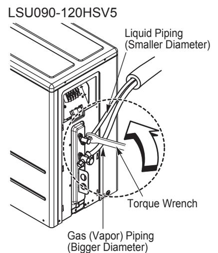
Figure 39: LSU180HSV5 Piping Connections. Figure 40: Pipe Attachment.
