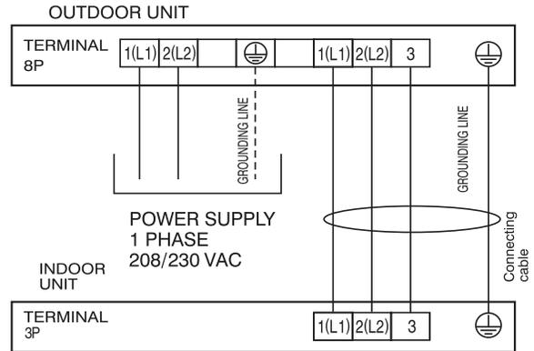
Figure 80: Typical LA240HSV3 Power / Communication System Diagram For Wiring Lengths Up to 130 Feet.
