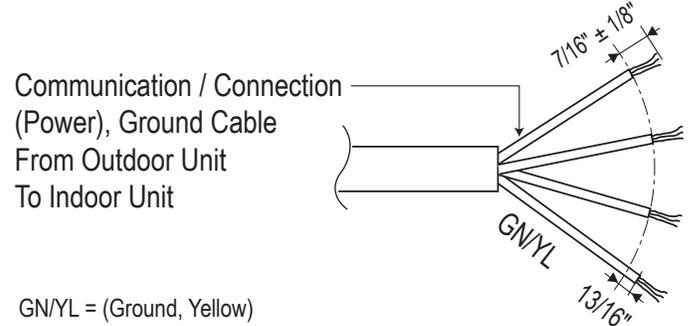
Figure 77: Single Zone Outdoor Unit to Indoor Unit Wiring and Communications Cable Diagram For Wiring Lengths GREATER THAN 130 Feet.
