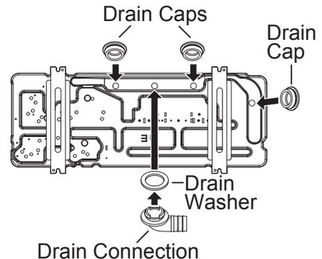
Figure 56: HSV5 Outdoor Unit Drain Hose Extension.
