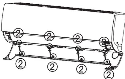
Figure 111: Snapping the Top Left and Right Sides (Step 4).
