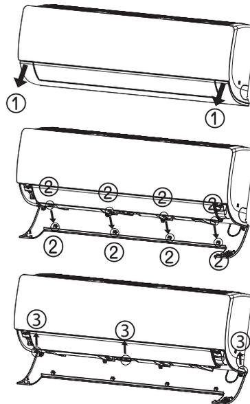
Figure 17: Removing the Bottom Cover (Appearances May Vary Depending on Indoor Unit Model).
