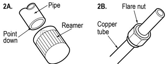
2B. Slide the flare nut onto the copper tube.
