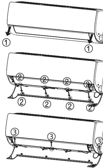
Figure 45: Removing the Bottom Cover, Alternate View.
