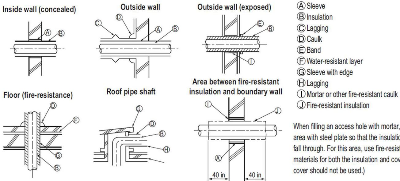
When filling an access hole with mortar, cover the area with steel plate so that the insulation will not fall through. For this area, use fire-resistant materials for both the insulation and cover. (Vinyl cover should not be used.)
