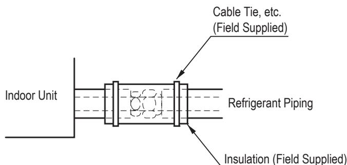
Figure 65: Typical Insulation Butt-Joint at Indoor Unit Casing.
