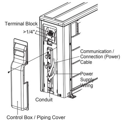
Figure 101: Accessing LSU180HSV5 / LAU240HSV3 Outdoor Unit Wiring Connections.
