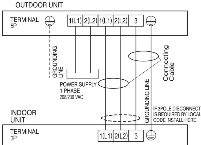
Figure 82: Typical LA180HSV5 Power / Communication System Diagram For Wiring Lengths GREATER THAN 130 Feet.
