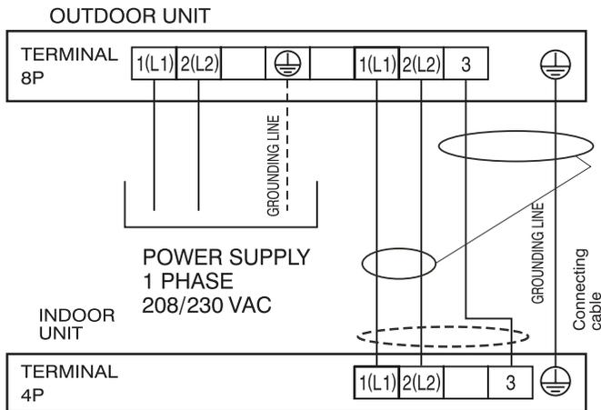
Figure 84: Schematic of a Single Zone System When the Wiring is GREATER THAN 130 Feet.
