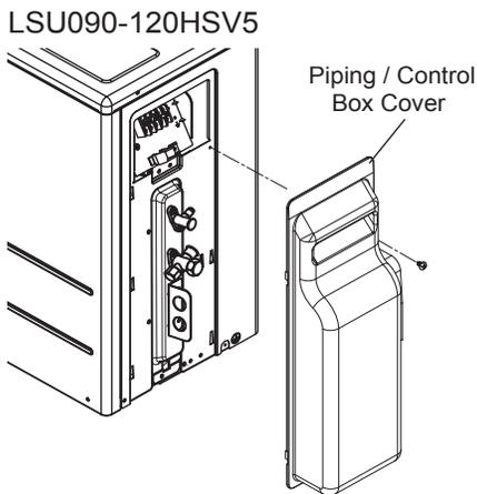
Figure 37: LSU180HSV5 Piping Cover and Control Box Cover Removal.
