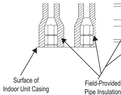
Figure 66: Typical Refrigerant Flare Fitting Insulation Detail.
