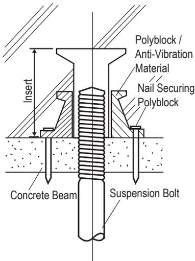
Figure 7: Close up of Bolt Attachment.
