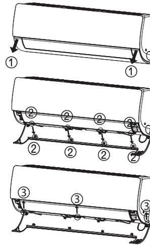
Figure 89: Removing the Bottom Cover (Appearances May Vary Depending on Indoor Unit Model).
