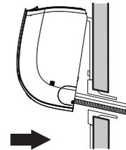
4. Carefully guide the refrigerant piping and drain piping through the access hole.
