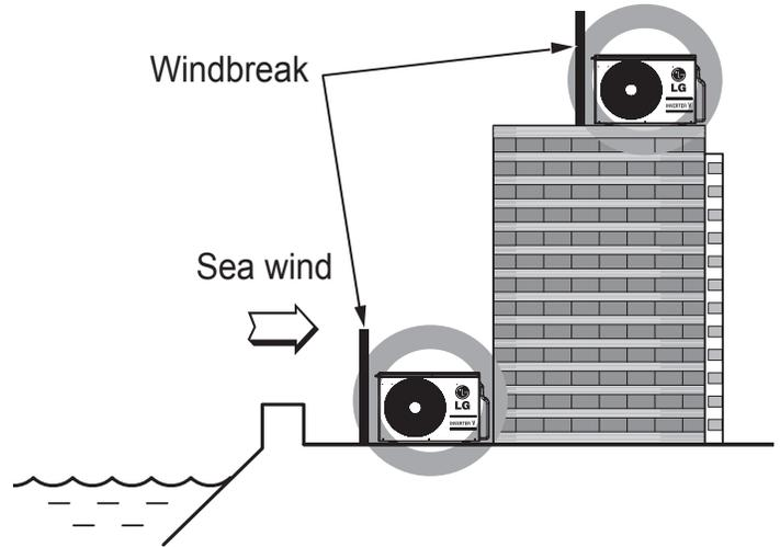
Figure 3: Placement Using Building as Shield.
