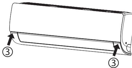
Figure 112: Checking that All Attachment Locations Are Secure (Step 5).
