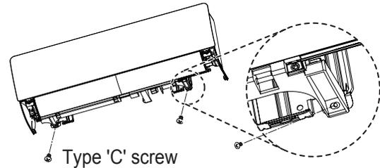
6. Finish the installation by completely securing the indoor unit to the installation plate using the factory-supplied two Type “C” screws at the locations indicated at right.
