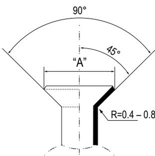
Flared Connection Dimensions / Tightening Torque.
