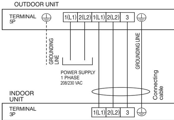
Figure 79: Typical LA180HSV5 Power / Communication System Diagram For Wiring Lengths Up to 130 Feet.
