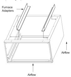
Fig. 6 - Use of Furnace Adapters
