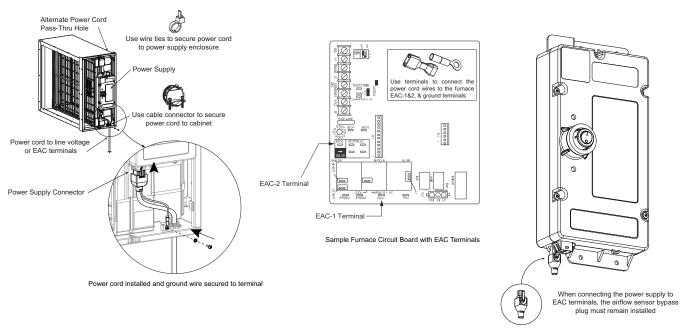
Fig. 9 - Infinity Air Purifier Electrical Connections
