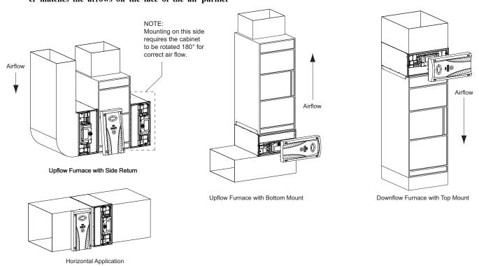
Fig. 3 - Infinity Air Purifier Cabinet Orientation
