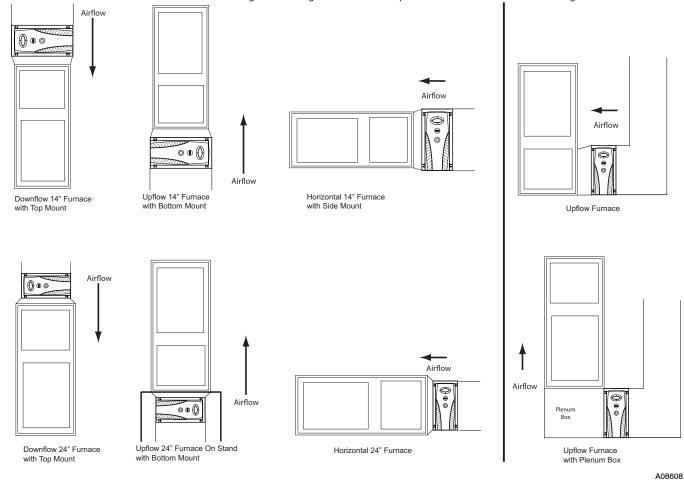
Fig. 4 - Infinity Air Purifier Cabinet Orientation with Transition
