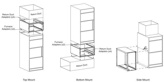
Fig. 5 - Mounting Infinity Air Purifier Cabinet
