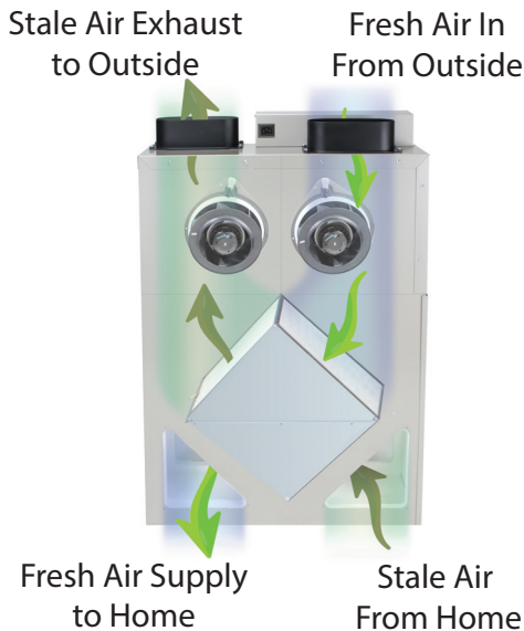
Fig. 4 - Airflow During Air Exchange
