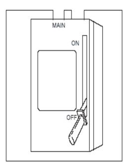
Fig. 1 - Main Electrical Disconnect
