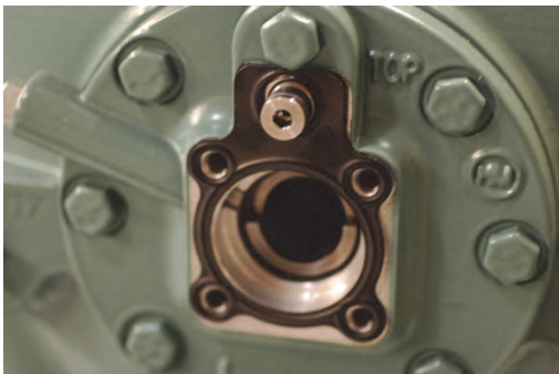
Fig. 18 — OPSS Sensor Block Gasket
