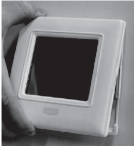
Fig. 11 - Attach Display to Backplate
