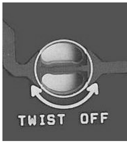
Fig. 1 - PCB Breakout Jumper
