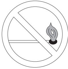
Fig. 3 - Do Not Light Burner with Match
