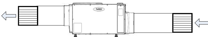
Figure 2 Dehumidifier Ducted Directly
