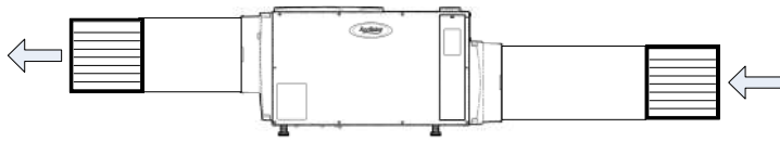
Figure 1 Dehumidifier Ducted Directly
