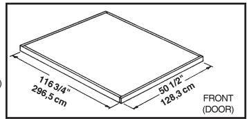
Note: Finished Slab dimensions, with lumber removed.
