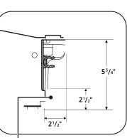
You must arrange the water supply line, power cable and drain hose in the space behind the dishwasher.
