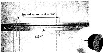
Level Hang Rail and mark holes 86.5" above floor that land on studs, then drill 1/8" pilot holes for screws.
