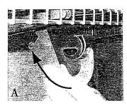
Install Rod Hanger into bottom of Bracket by tilting it backward until it locks in place.
