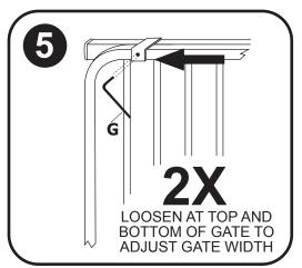
Set screws on top and bottom of gate to extend gate. LEAVE SHIPPING TABS IN PLACE TO NOT MAR GATE FINISH. You will remove shipping tabs during final tightening.
