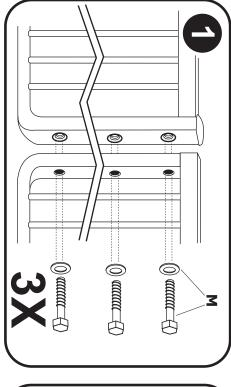
Using bolts and washers included, attach extension to hinge side of gate.
