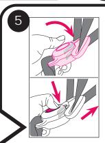
Unbuckle harness by tilting top of buckle down, press top of red button, and pull tongues out of buckle.
