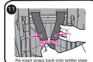
Turn page over to finish the rest of the assembly Steps 12 to 20 for the buckle replacement.
