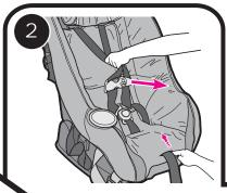
To loosen straps, lift lever and pull harness straps.
